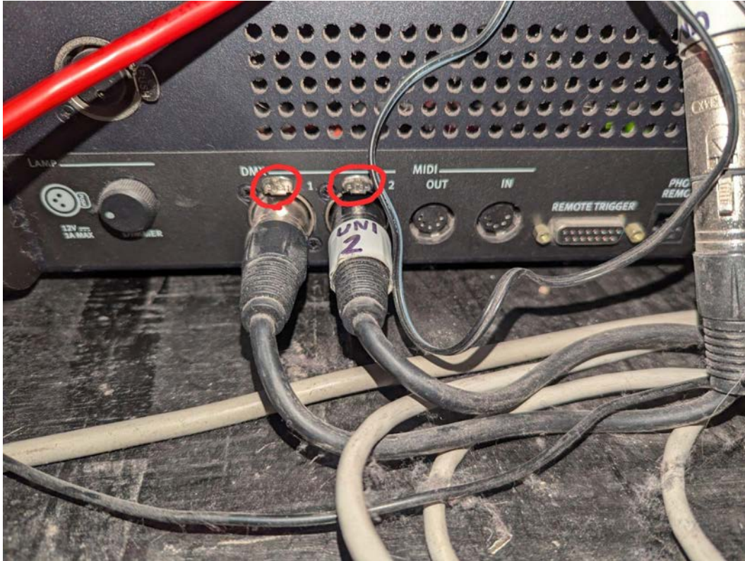
Alternative view of the DMX cables with release levers highlighted
