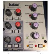
which bank you are looking at. Once selected, the program takes about a second to load, and parameters within each program can be adjusted with the 'Adjust' knobs.
