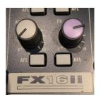
The reverb going to the output (i.e. coming through the speakers) is controlled by the 'EFFECTS RETURN' knob, which is the right hand knob directly below the 'Lexicon' logo. You can send the reverb to *either* 'MIX' *or* 'SUB' speakers. Turn this up gently while someone is talking into the mic and see how this sounds. Adjust parameters until you get the desired effect.
